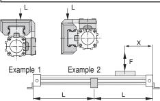
Number of supports needed (n) given that the cylinder is fixed on the ends.
