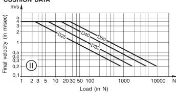
The velocities indicated in graph (I) represent **final velocities**. To properly determine the inertial forces for cushioning, it is important to know the **final velocity**.
